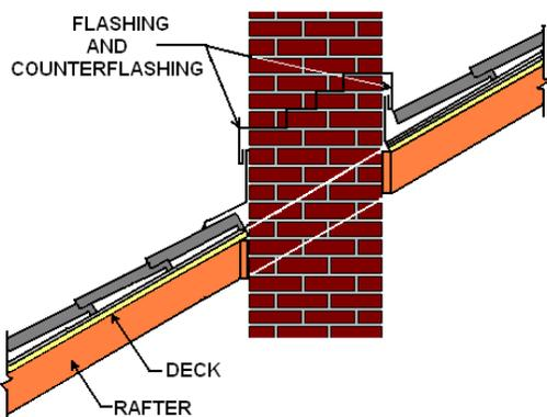
**Sidewall flashing (26-Gauge)**
